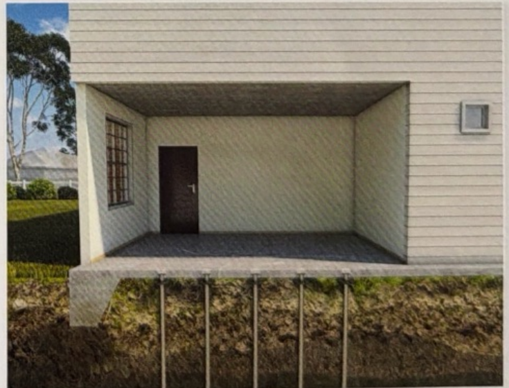
AFTER: Slab Pier support
